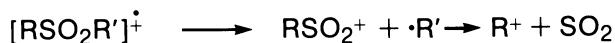
Figure 30. Poly(butene-1-sulfone), PBS. The radiochemical decomposition pathway via a radical cation is proposed by O'Donnell.
